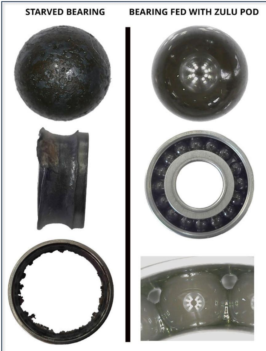
Hardware **failure** and **performance degradation** from a simulated loss of lubrication event was **mitigated** by a product delivering minimum lubrication over time - increasing technology maturation to **TRL 5**.
